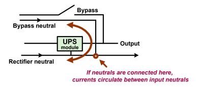
While these circulating currents are a minor nuisance when the bypass and rectifier come from the same source, this can be a hazard if the two input neutrals come from different sources. The connection of two independently derived neutral sources together is universally not permitted by law. The insertion of a transformer in series with one of the two sources solves this problem. Whenever a dual mains UPS is supplied by separately derived neutral
