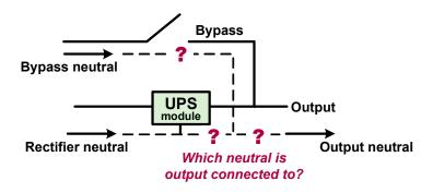
Since switching between neutrals supplying an IT load creates a momentary open-neutral condition which can be hazardous or destructive, the neutral to the critical load should never be switched. This means if two alternate sources are combined in the UPS, they must have their neutral wires permanently connected to each other. However, connecting the input neutrals together to the output neutral can create circulating currents between the input neutrals as shown in **Figure 5**.
