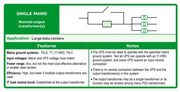
Another option for large data centers is to add an input transformer to the "single mains with remote output transformer" arrangement, to allow for use with very poor mains grounding systems or a mains supply with an incompatible grounding system, but this would be an uncommon situation.
