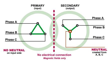
The primary, or input, is on the left and three power phases are applied to the transformer windings (green lines) that are connected in the "delta" configuration as shown by the triangular shape.
